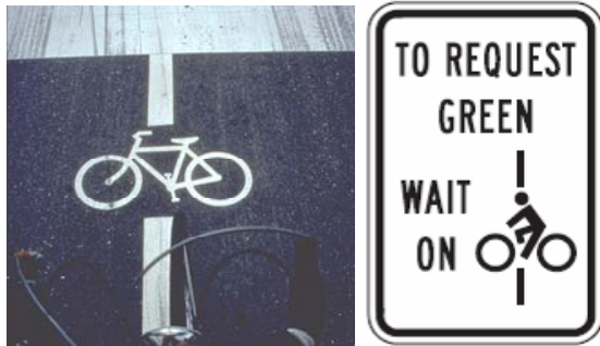
Figure 8. Signal activation marking and sign.
