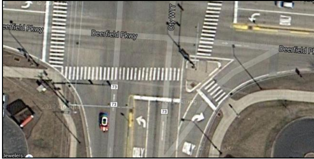
Figure 2.5. Right-turn corner island and high-visibility continental crosswalks, southeast corner of Deerfield and Weiland
