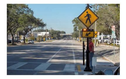
Figure 2.13. Rectangular Rapid Flashing Beacon. Courtesy FHWA.
