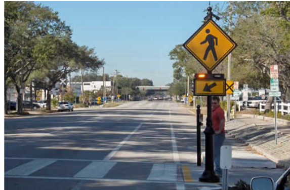
Left, top to bottom: W11-1, W16-9P, W16-7P. Center: R1-5B. Right: Rectangular Rapid Flashing Beacon
