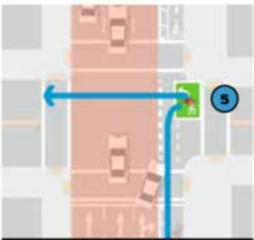
Crosswalk Setback Configuration Wider corner radii, set back pedestrian crossing, and/or narrowed bikeway space, provides opportunity for queue box.
