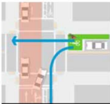
Bike Box Configuration Bicyclists yield to pedestrians. Not recommended in areas with high pedestrian volumes.
