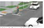
A bicycle forward stop bar can reduce the minimum acceptable gap by one second per cycle of the street.
