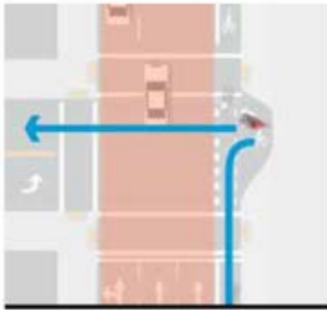
T-Intersection "Jughandle" Sidewalk Configuration
