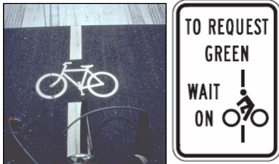
Figure 2.12. Signal activation marking and sign.
